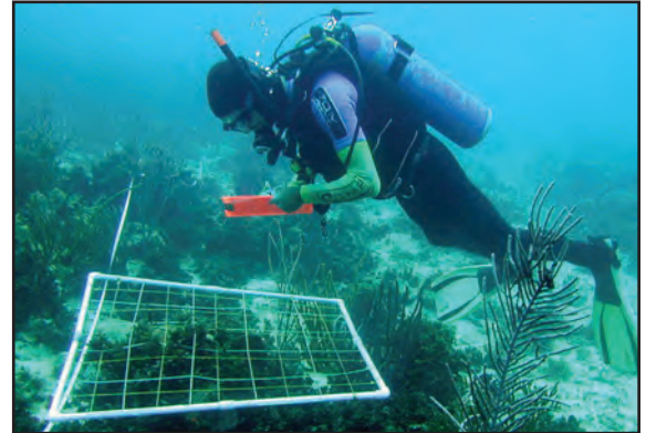
Figure 2.1. NOAA diver recording benthic habitat composition within the randomly placed 1 m 2 quadrat along the belt transect.
