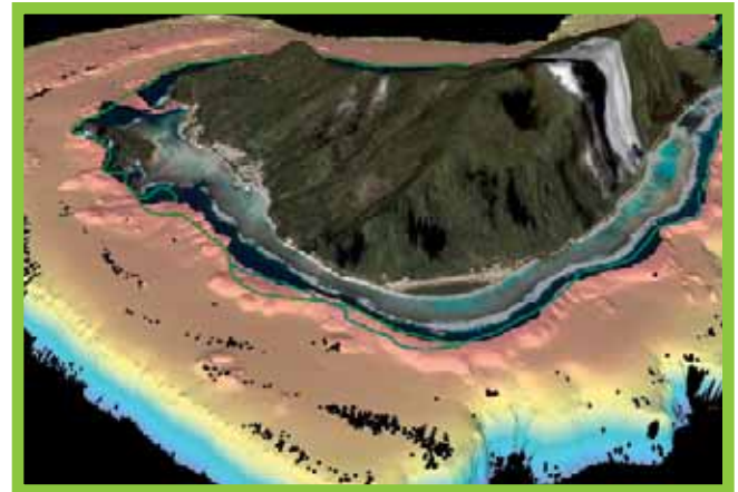
Map products depict water depths and seafloor features in nearshore areas around the island of Ofu in American Samoa. Black areas indicate data "holidays" or areas for which no information was collected.
