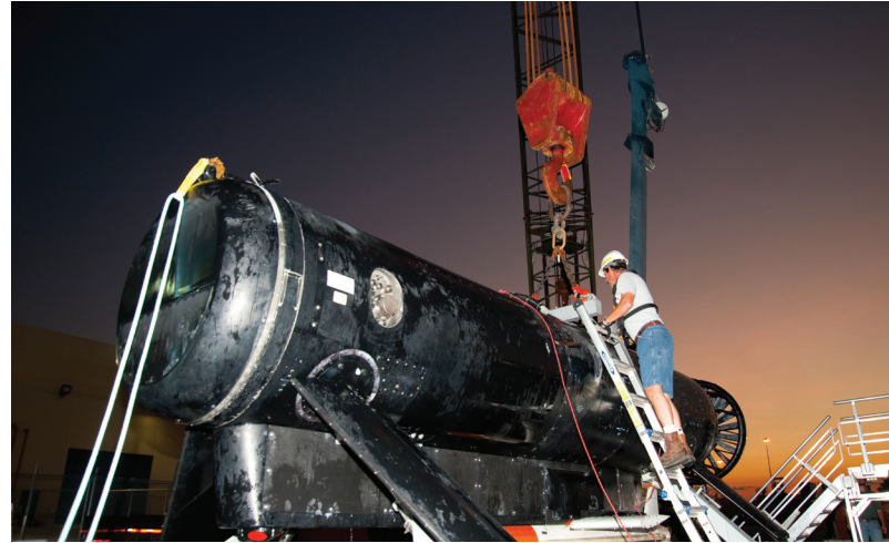
Naval Surface Warfare Center Panama City engineers recover the Remote Multi-Mission Vehicle, part of the Mine Countermeasure mission package, following end-to-end tests. U.S. Navy photo by David Sussman.
