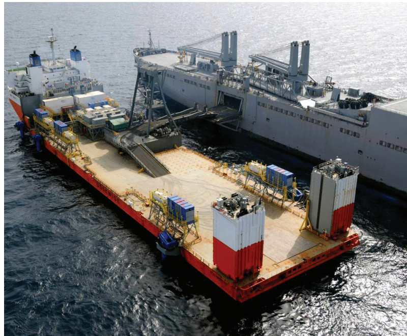
Using a surrogate mobile landing platform (MLP) ship (M/V Mighty Servant 3 , shown left), the Navy conducted an at-sea demonstration, transferring vehicles from the “MLP” to a large/medium-speed, roll-on/roll-off (LMSR) ship (USNS Soderman , shown right) using the Test Article Vehicle Transfer System (TAVTS). TAVTS—the grey bridge structure spanning the two vessels—allowed personnel and vehicles to transfer between the ships in both high and low sea states. U.S. Navy photo.
