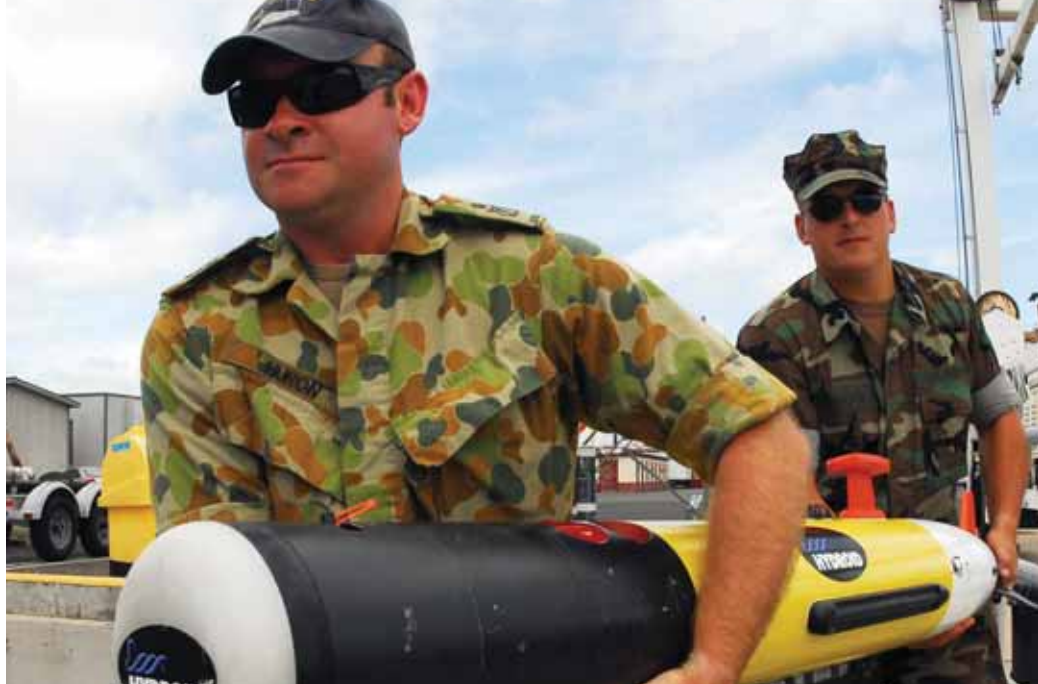
Sailors carry a Remote Environmental Measuring Unit (REMUS) during the Honolulu Harbor experiment. Photo by MC2 John W Ciccarelli Jr.
