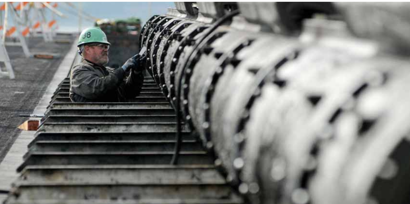
A Puget Sound Naval Shipyard worker cleans a section of a steam-powered catapult track aboard USS Abraham Lincoln (CVN 72). Photo by MC2 James R. Evans
