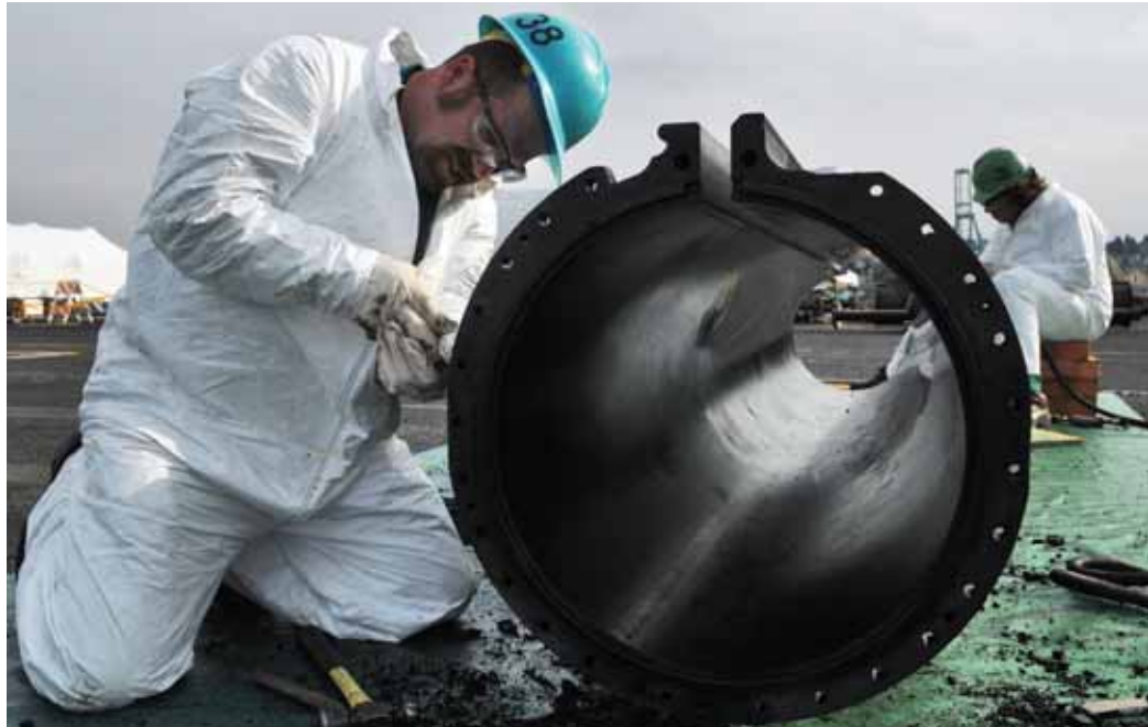
Darren Schmittler cleans a section of a steam-powered catapult track aboard USS Abraham Lincoln (CVN 72) at Puget Sound Naval Shipyard. Photo by MC2 James R. Evans
