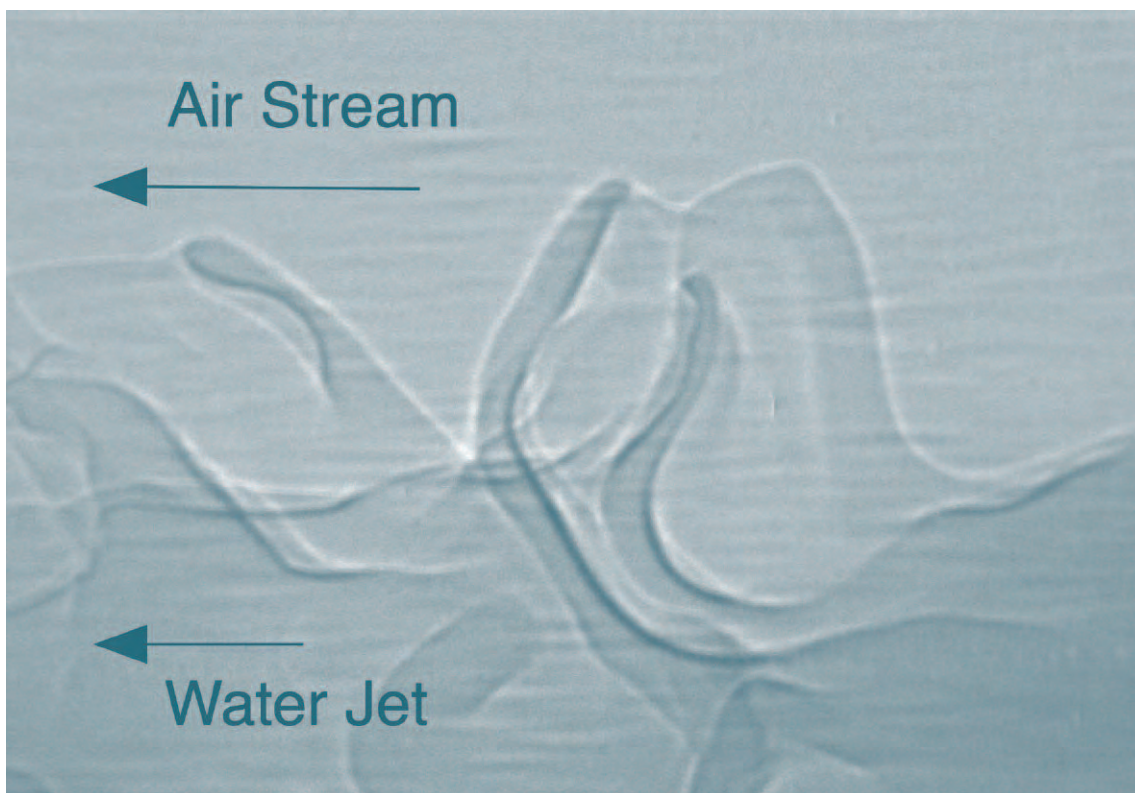
Fig. 1. X-ray phase-contrast image showing membranes entrained by the streaming air (at 90 m/sec) and separating from the main water jet. The exposure time is 472 nsec, and the image size is 1.4 \times 1.7 \text{ mm}^2 .
