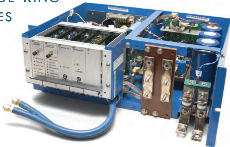
A storage ring DC-to-DC converter.
