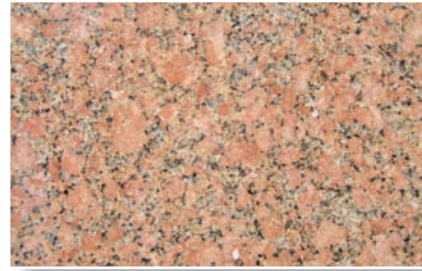
Figure 1-3. Cut and polished granite showing pink and white quartz crystals and black mica.
