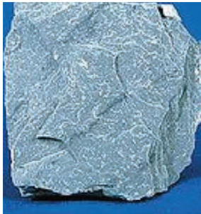
Figure 1-6. Slate, a fine-grained, foliated, metamorphic rock that was formerly shale. (Courtesy of USGS Rock Library.)
