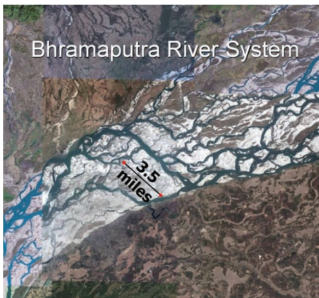
Figure 3-20. Closer Image of Braided River Fluvial Depositional System showing the area in red in previous figure. (Google Earth Image modified from Hannes Leetaru, 2009.)
