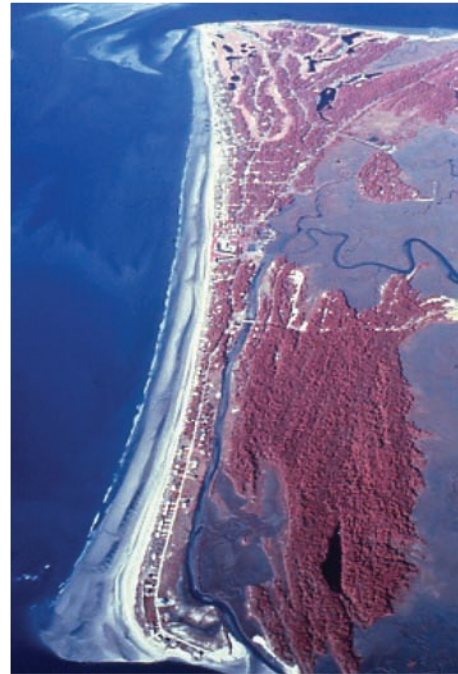
Figure 3-13. Strandplain Deposit along the South Carolina Coast (infrared satellite image). Note the linear sand ridges building toward the ocean as the strandplain builds through sand brought by long-shore currents. The layered appearance results from the accumulation of new strandlines. (Hayes, 1989.)
