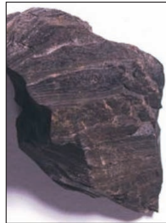
Figure 1-13. Shale with parallel bands or layers. (Courtesy of USGS Rock Library.)
