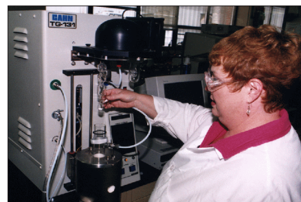
Solid Sample Being Loaded into Thermogravimetric Analyzer
