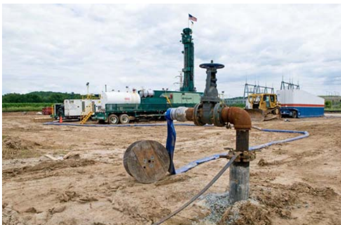
MRCSP CO 2 injection testing in the Mt. Simon Sandstone deep saline formation.
