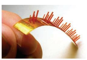
**The right bent.** The artificial hair cells are only 500 to 700 micrometers long and can be adapted to function as both vibration and tactile sensors.
