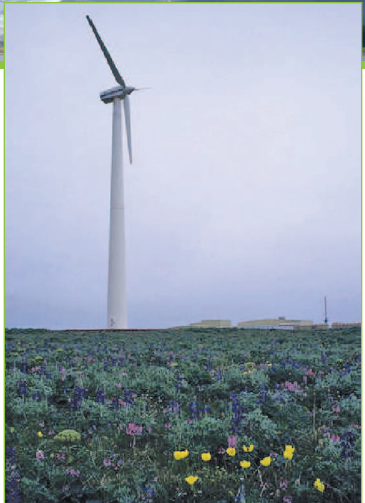
Vestas 225-kW wind turbine on the St Paul. Ed Linton, Northern Power Systems/PIX10597.
