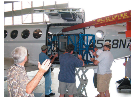
Installation of the IIT ACCLAIM instrument already installed its associated pallet into the NASA Langley UC-12B aircraft prior to AID for ASCENDS.
