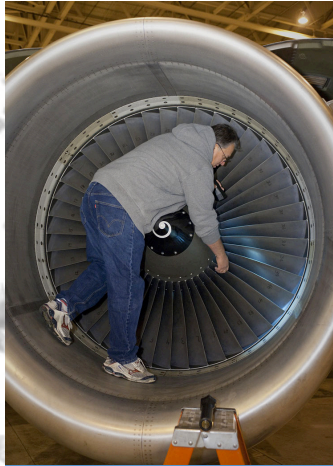
Enrique Hernandez inspects turbine blades of DC-8 engine.
