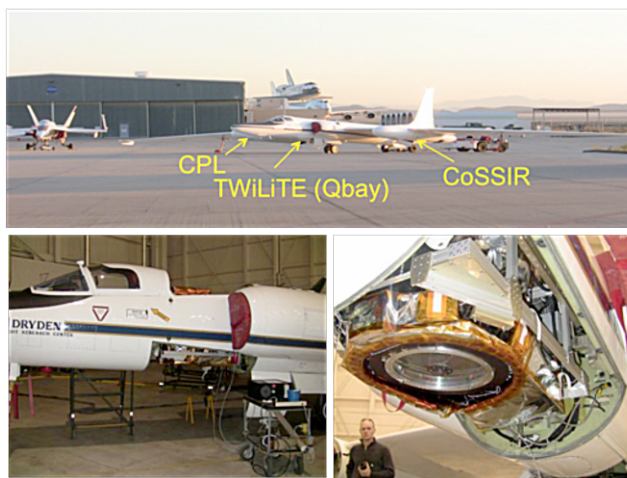
Figure 23: ER-2 carrying CPL, TWiLiTE and CoSSIR for an instrument test mission.
