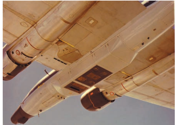
Figure 53 WB-57F Showing Universal Pallet System (UPS)
