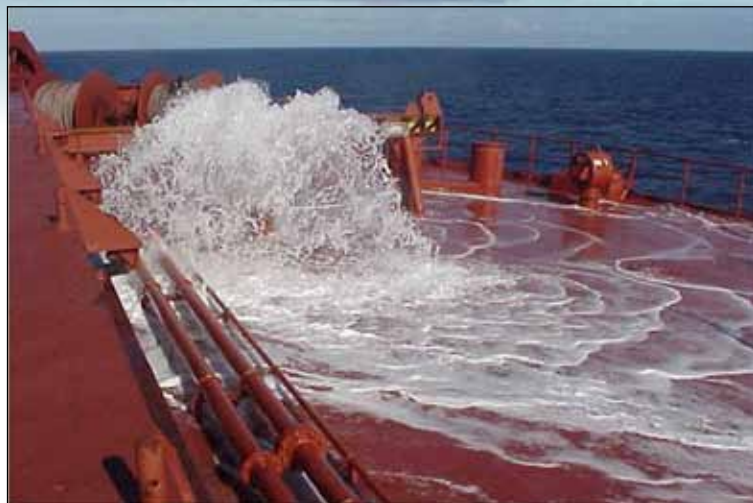
▲ Water overflowing from a ballast tank deck hatch during ballast water exchange at sea.
