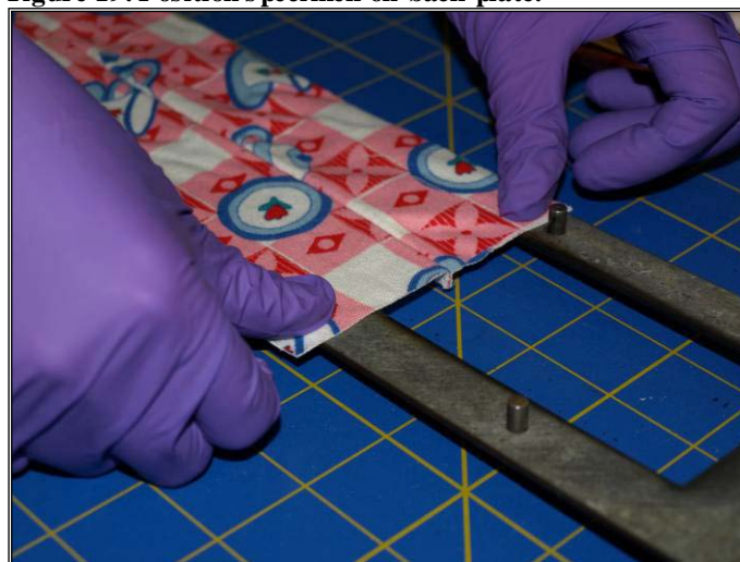
Figure 20. Position seam specimen on back plate.
