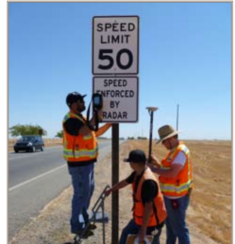
Team members check the retroreflectivity of a road sign during a traffic management controls survey. Photo courtesy of Sacramento District, U.S. Army Corps of Engineers
