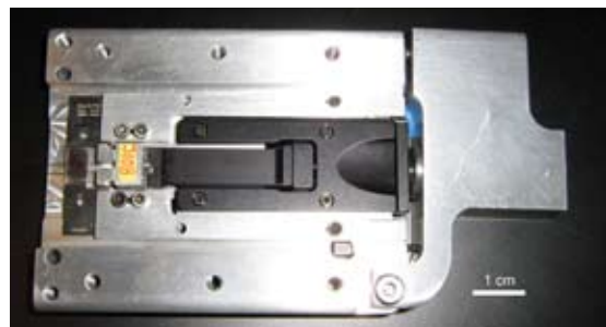
The SafePort housing structure contains the components that integrate the contaminant-specific microchip (black) with the external environment to sample and analyze water in the field. Photo by Travis King
