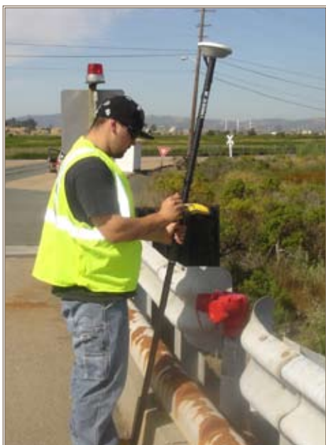
A survey crew member uses a handheld GPS device to record a feature. Photos by Mike Haskell
