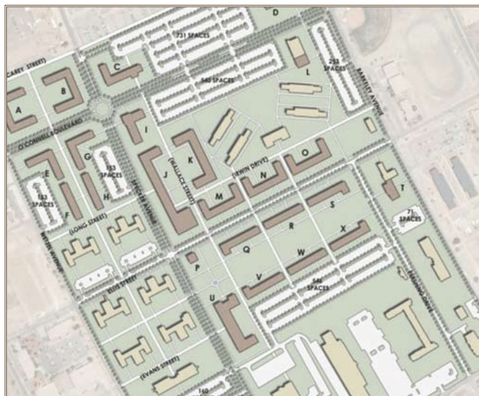
This energy-effective area development plan involves compact development, interconnected streets and narrow buildings. Graphic courtesy of Jerry Zekert
