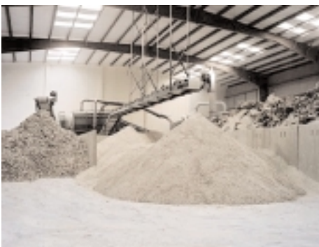
Taylor Recycling facility wallboard recovery operation.
