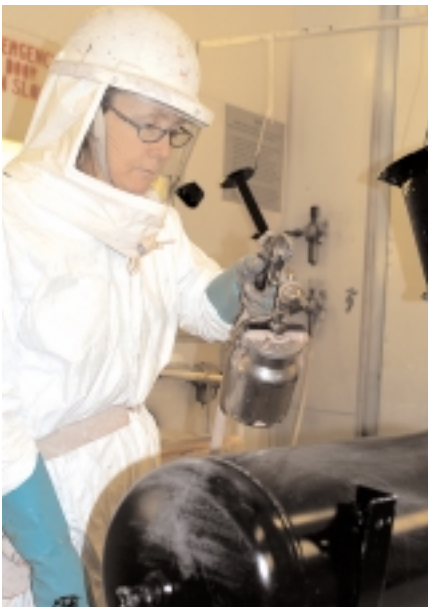
Tobyhanna painter Donna Sheebey-Frizzie uses low Volatile Organic Compound (VOC) paint on a component from an Air Force Range Threat System maintained at Tobyhanna Army Depot.
