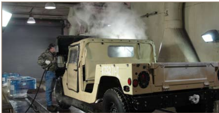
A LEAD employee cleans a vehicle with a high-pressure closed-looped system, which conserves water and minimizes discharge to the industrial wastewater plant. Photo by Todd L. Johnson, LEAD Environmental Office
