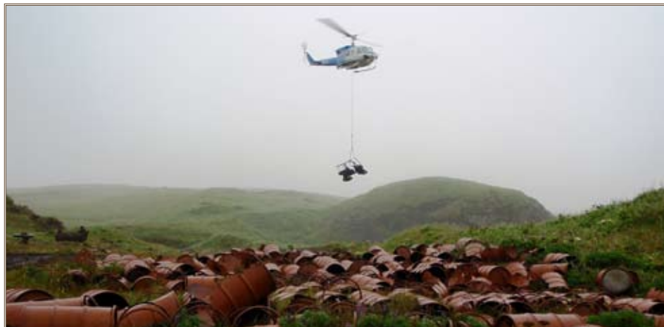
On Tanaga Island, a helicopter sling-loads a utility vehicle that was used for site access several miles over a debris field, one of the site conditions that made access difficult. Photo by Mike Macmillan, USACE Alaska District
