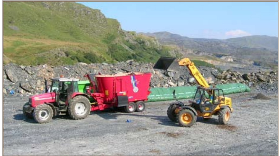
Workers prepare an EcoPod, a composting method that CERL studied at two installations, to receive material. Photos courtesy of AgBag Systems, U.K.
