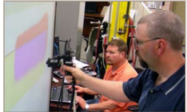
Blue Grass Army Depot instructor Chris Adams shows employee Tim Hampton through a virtual-reality training simulator the correct thickness to apply CARC, which will help Blue Grass generate less waste and save paint. Photo by Mark Henry, Blue Grass Army Depot
