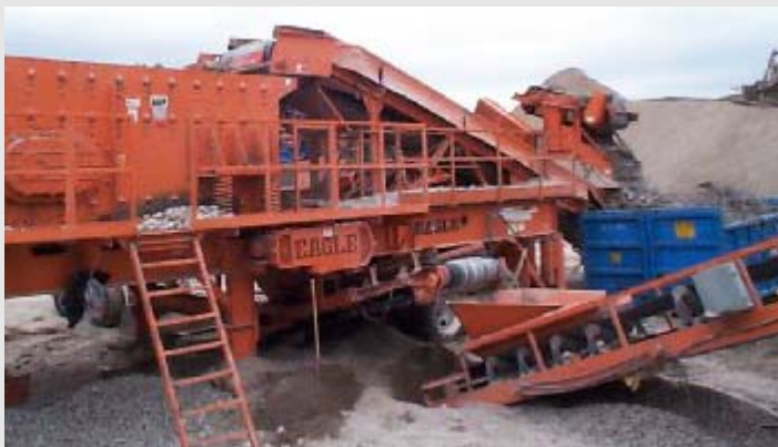
Eagle crusher used to process concrete at Fort Ord.
