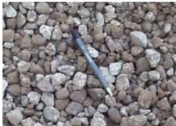
Concrete debris after removal from the demolition site and after crushing into aggregate.
