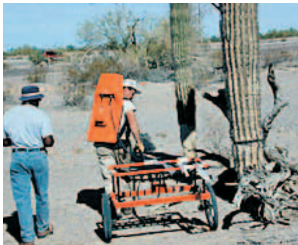
A team tests a prospective UXO detecting system on the Standardized UXO Technology Demonstration Site on Yuma Proving Ground, Ariz. USAEC file photo.
