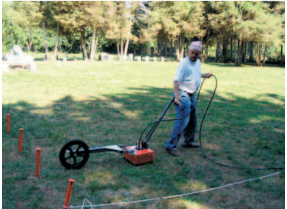
Ground penetrating radar being used by Fort Drum's cultural resources staff to locate burial sites at Sackets Harbor (NY) Military Cemetery. Photo courtesy of Fort Drum
