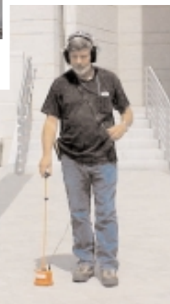
Ron Vanasco uses the electronic leak detector.
