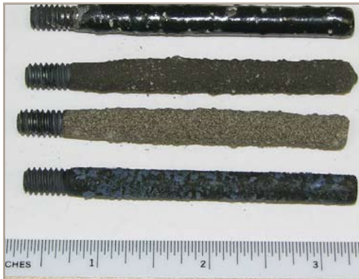
Engineer Research and Development Center has a patent pending for a novel vitreous enamel coating that prevents rebar corrosion. Photo courtesy of ERDC
