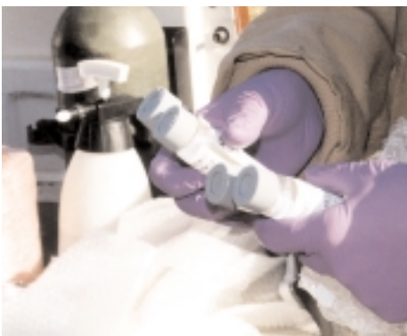
Vials used for groundwater samples are collected at Fort Leavenworth, Kansas, for laboratory analysis. Volatile organic compounds are analyzed on a regular basis and the results help determine the effectiveness of the remediation.
