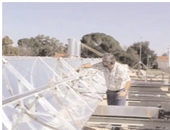
Technician shown checking the tracking module. Sun-tracking sensors detect concentrated sunlight reflected from the rims of the parabola.
