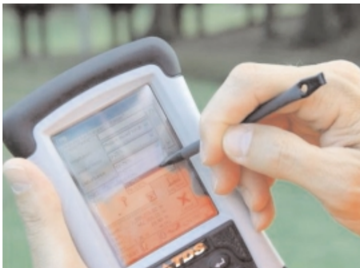
Field observations and other data can be manually entered onto project-specific, customized forms, which are pre-loaded on ARMS™ as required.
