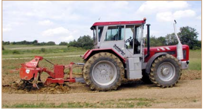
A tractor pulls specially developed decompaction equipment that loosens the soil but does not destroy vegetation, both of which are very important for the prevention of surface water erosion. Photo courtesy of Manfred Rieck
