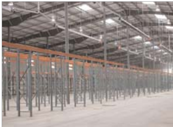
The pallet rack in the new pallet handling facility will hold 10,000 pounds.
