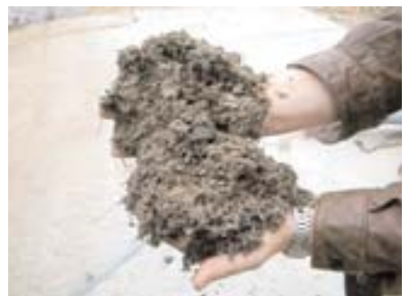
Organic material, or fluff, produced by the WastAway System.
