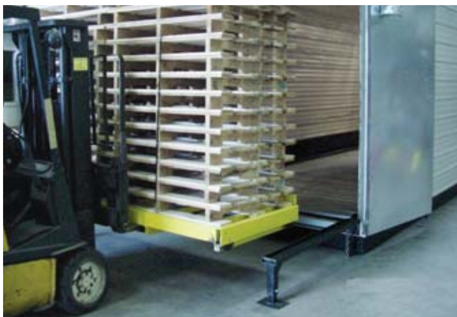
Rapid pallet loading system at the thermal pest management chamber
