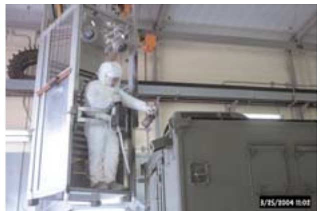
The Mobile Zone cab provides a full four-degree of movement, allowing workers to move around the equipment to be painted.
