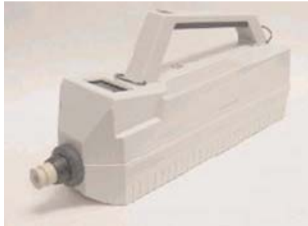
The VT2 is a hand-held explosive detector.
