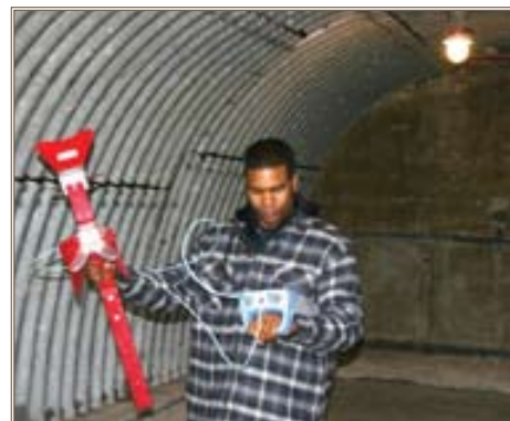
Several tests, such as radiofrequency sensing, were used to validate EOP's safety in bunkers. Photo courtesy of ERDC-CERL
