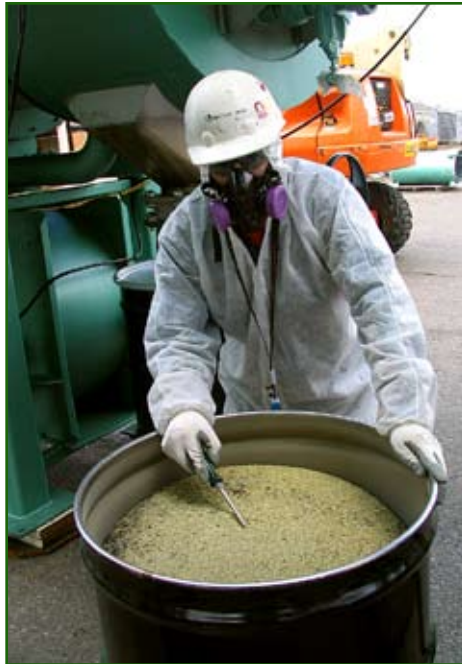
Nick Bostwick, waste technician with ARI Technologies, examines the material discharged from the primary combustion chamber. Photo by Brendalyn Carpenter.
