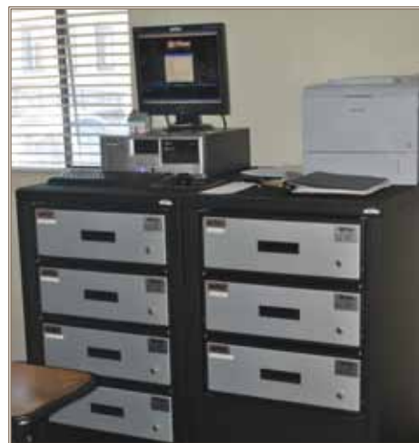
An automated key system holds and keeps track of keys for 10 barracks at Fort Irwin. Photo by Sgt. 1st Class James Elliot, noncommissioned officer in charge, SSSHO.
