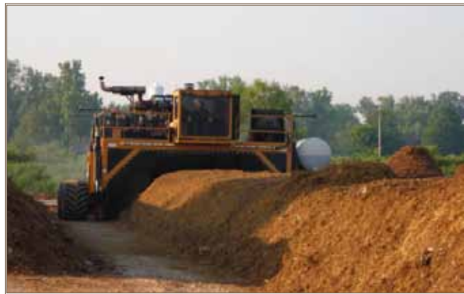
A worker uses windrow composting to treat contaminated soils at Plum Brook Ordnance Works. Photo courtesy of Engineer Research and Development Center
