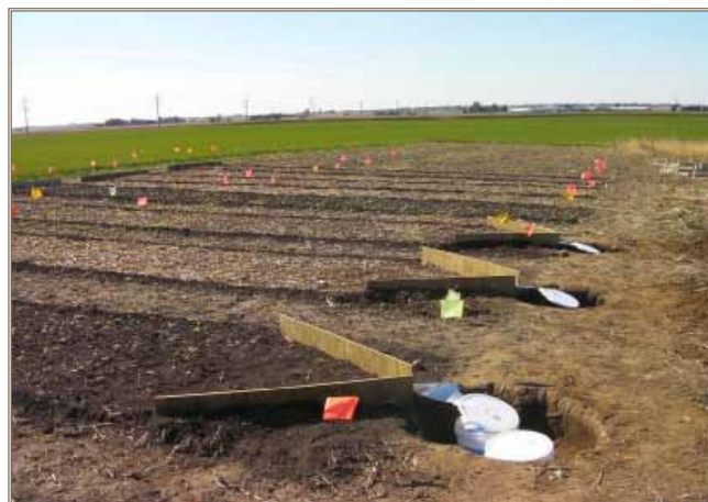
CERL evaluates composted mulch erosion control blankets in the field. Photo courtesy of ERDC
