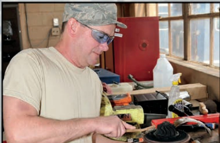
Tech. Sgt. Robert Snow, 181st LRF, cleans a Garrett Turbo off a Ford diesel truck. Photo by Master Sgt. John Day
