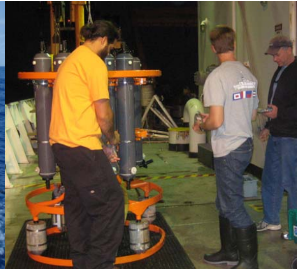
Collecting seawater samples from the CTD
