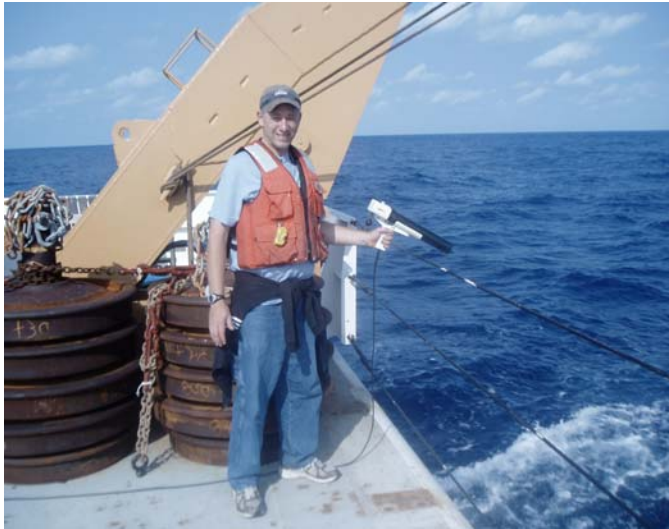
Here I am deploying an XBT.
