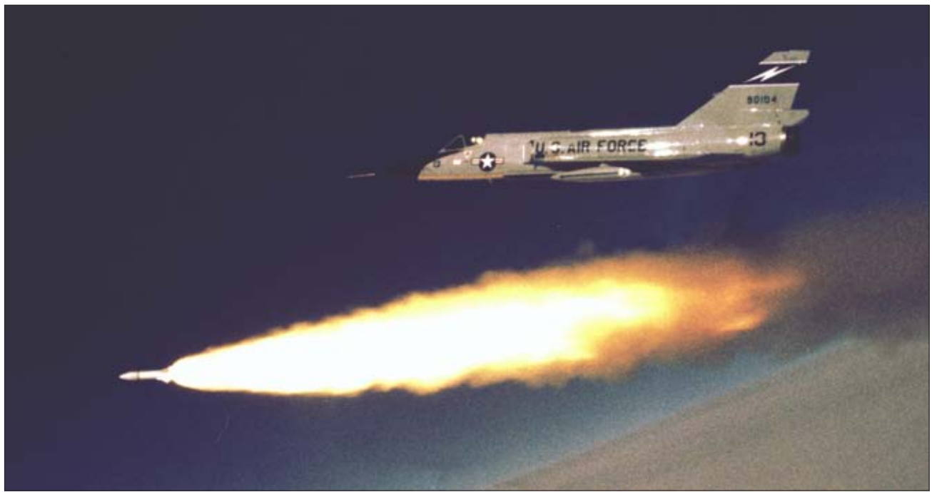
A 125FIG F-106 Delta Dart fires a AIR-2A “Genie” rocket with a simulated W-25 nuclear warhead at an unmanned drone.
