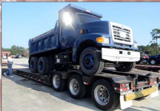
A dumptruck loaded on a removable gooseneck lowboy trailer. The removable gooseneck makes loading and unloading the trailer much easier and safer.
