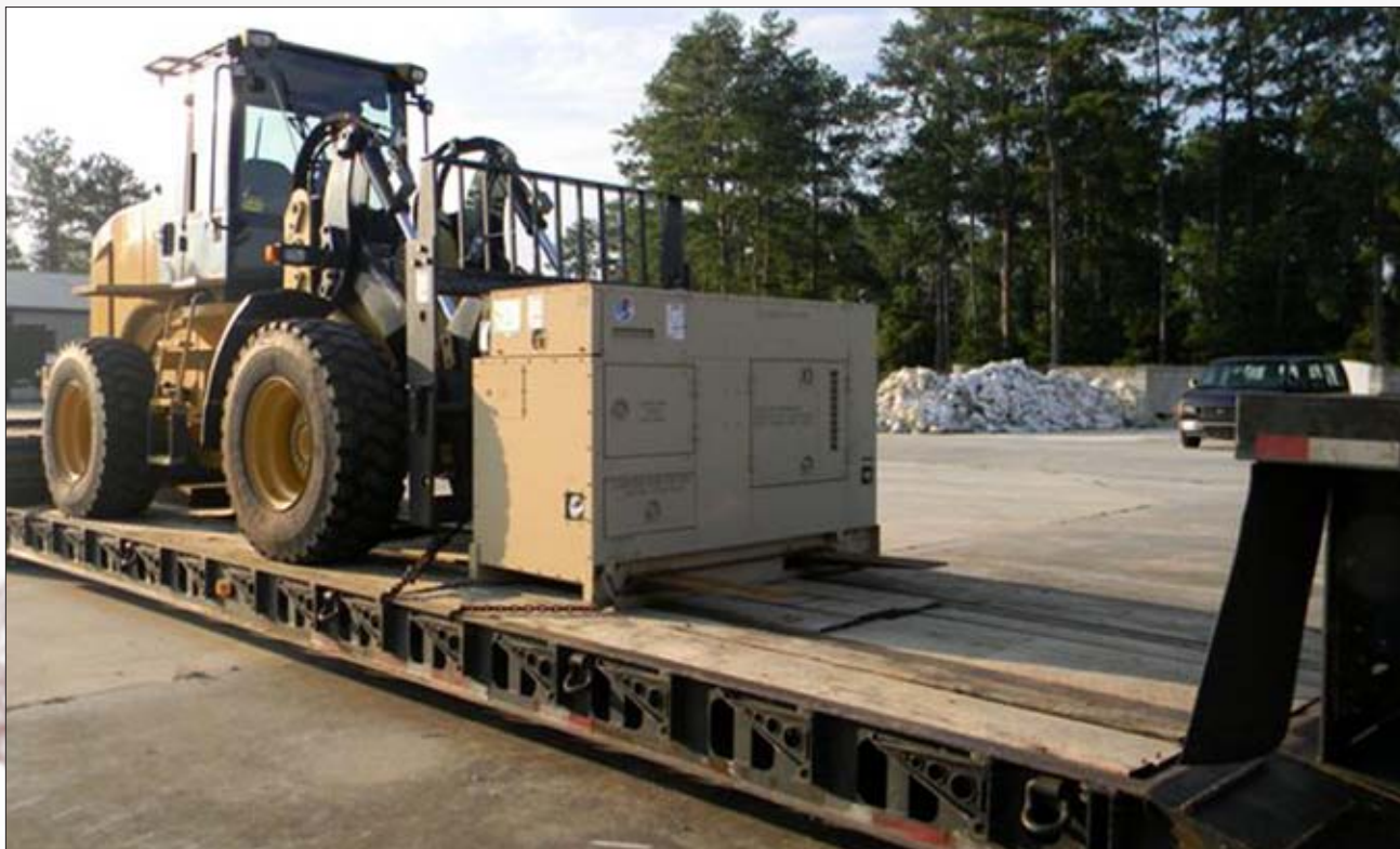
A 10K adverse-terrain forklift with a generator is loaded on a lowboy trailer. The forklift is used for loading and unloading palletized equipment up to a 10,000 pound limit.
