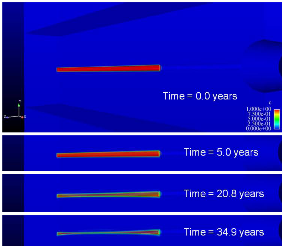
Figure 2.4-10. Normalized or Scaled Concentration of ^{137}\text{Cs} near the Waste as a Function of Time
