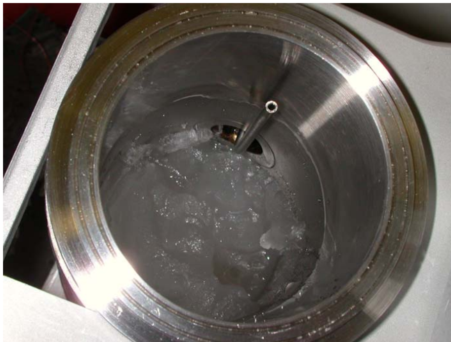
Figure 10. (Upper) R141b hydrate slush formed by 2 wt.% NaCl solution at 5°C in a stirred batch reactor. The elapsed time for this experiment was approximately 1000 seconds. (Lower) Appearance of R141b clathrate hydrates formed at 1°C in 2 wt.% NaCl solution.
