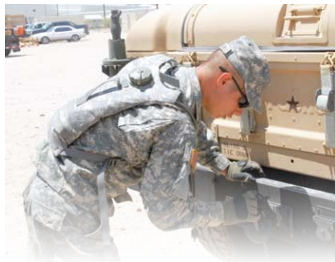
Pfc. Jared M. Blankenship, a truck driver with Company A, 701st Brigade Support Battalion, 4th Infantry Brigade Combat Team, inspects the trailer hitch during a pre-maintenance check and service of his Humvee at the National Training Center.
