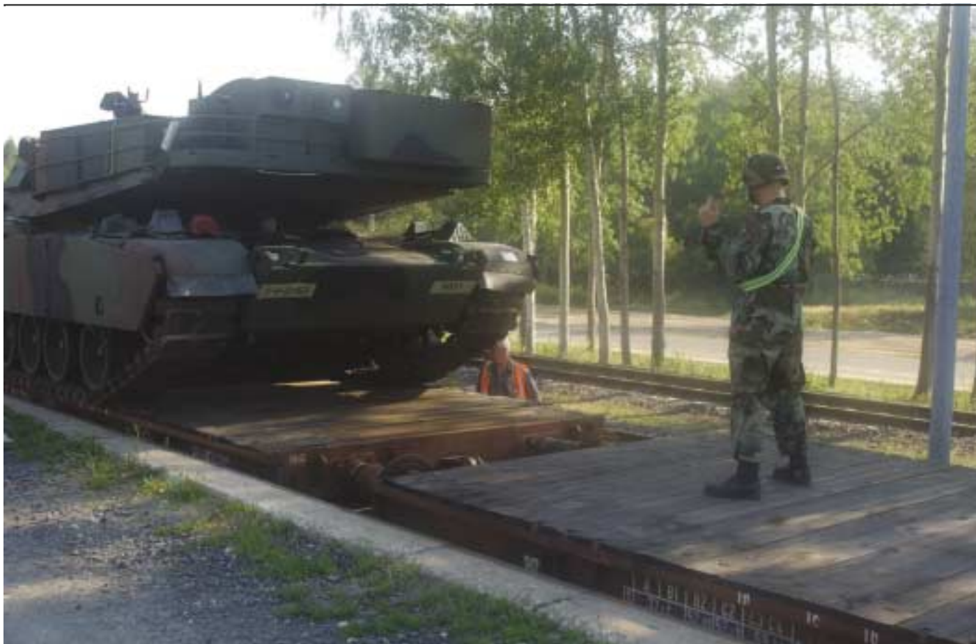
A 3rd Brigade Soldier ground guides an M1A1 Abrams tank as part of the railhead operations in Vilseck.
