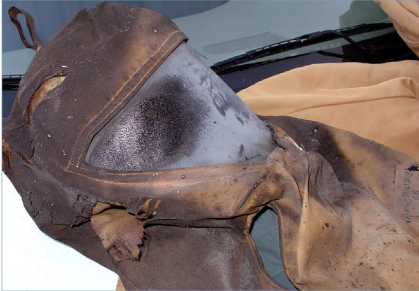
Figure 1-2. Damaged flash hood
