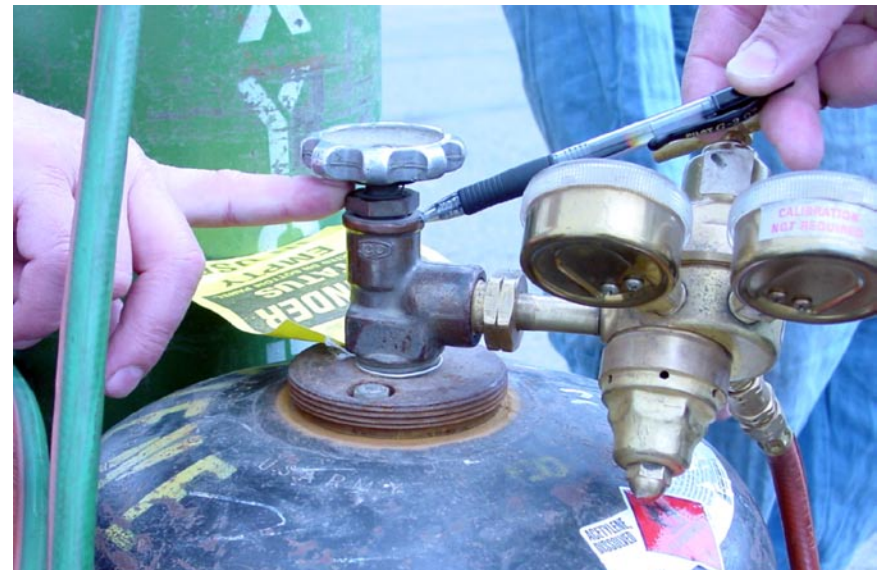
Figure 2-5. Fire originated between the isolation valve and packing nut
