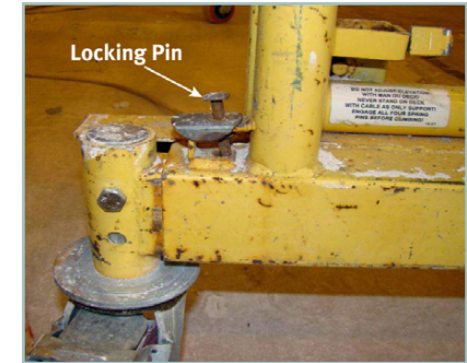
Figure 2-3. Example of locking pin not fully engaged
