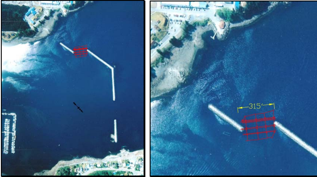
Figure 7. Alternative 4 closes the gap between the existing main and south breakwaters – drawing not to scale.
