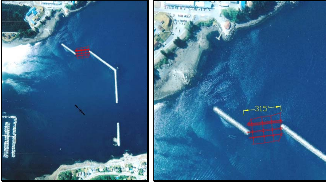
Figure 1. The recommended corrective action closes the gap between the existing main and south breakwaters – drawing not to scale.
