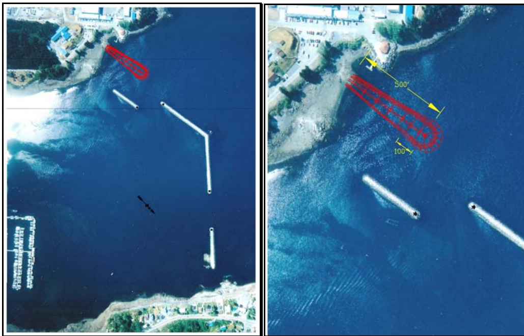
Figure 1. Alternative 1, stub breakwater, would extend from the Japonski Island shore northward to form a 100-foot overlap with the south breakwater—drawings not to scale.
