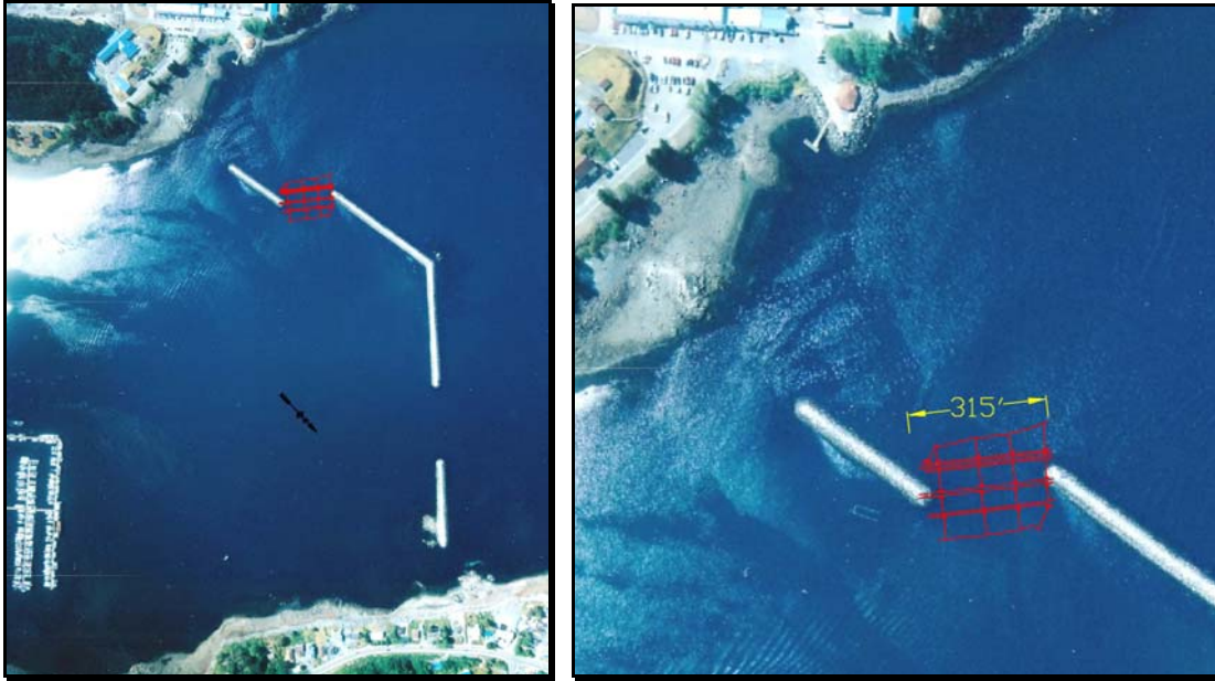
Figure 4. Alternative 4 closes the gap between the existing main and south breakwaters – drawing not to scale.
