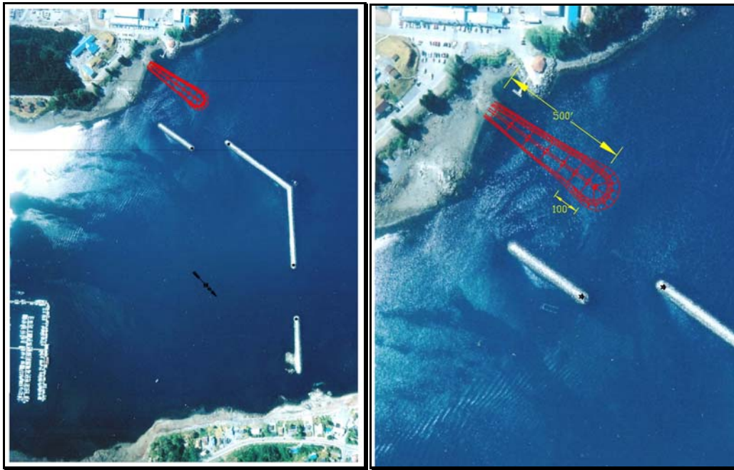
Figure 4. Alternative 1, stub breakwater, would extend from the Japonski Island shore northward to form a 100-foot overlap with the south breakwater—drawings not to scale.
