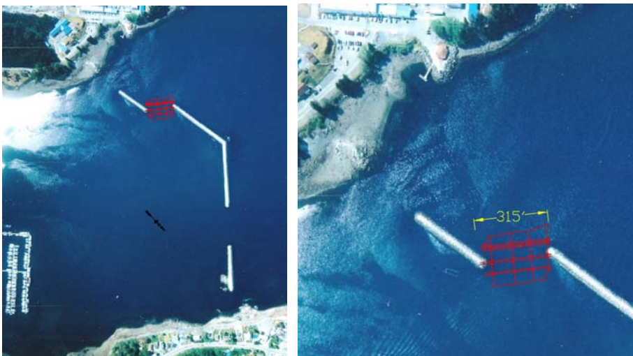
Figure 33. Alternative 4 - Breakwater Closure between Main and South Breakwaters – drawing not to scale.
