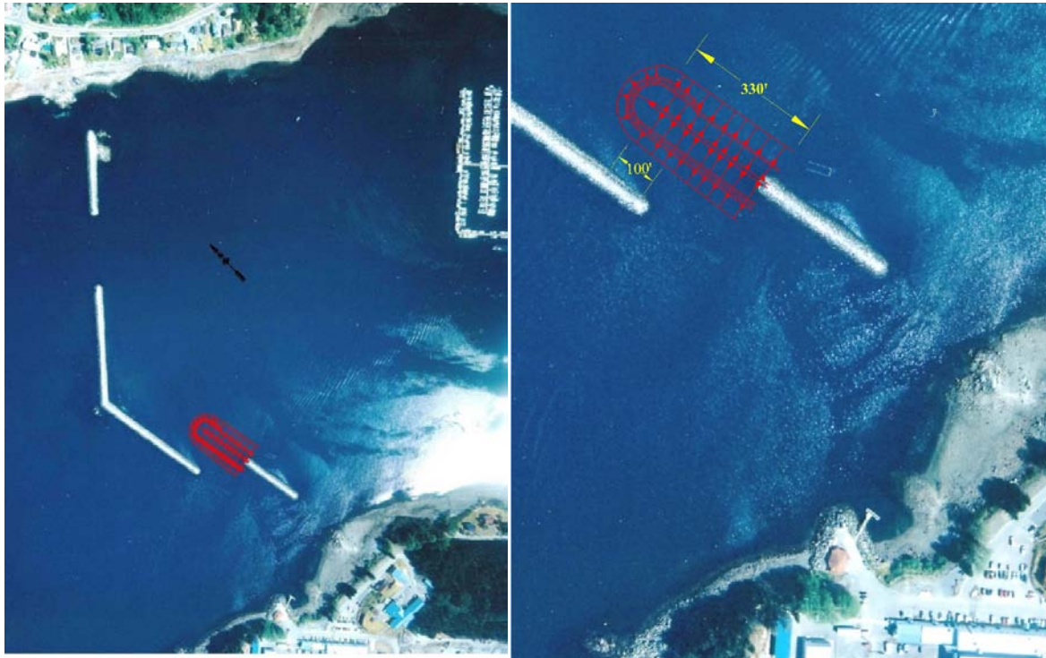
Figure 27. Plan 2. Breakwater overlap inside overall and close up view – drawing not to scale.
