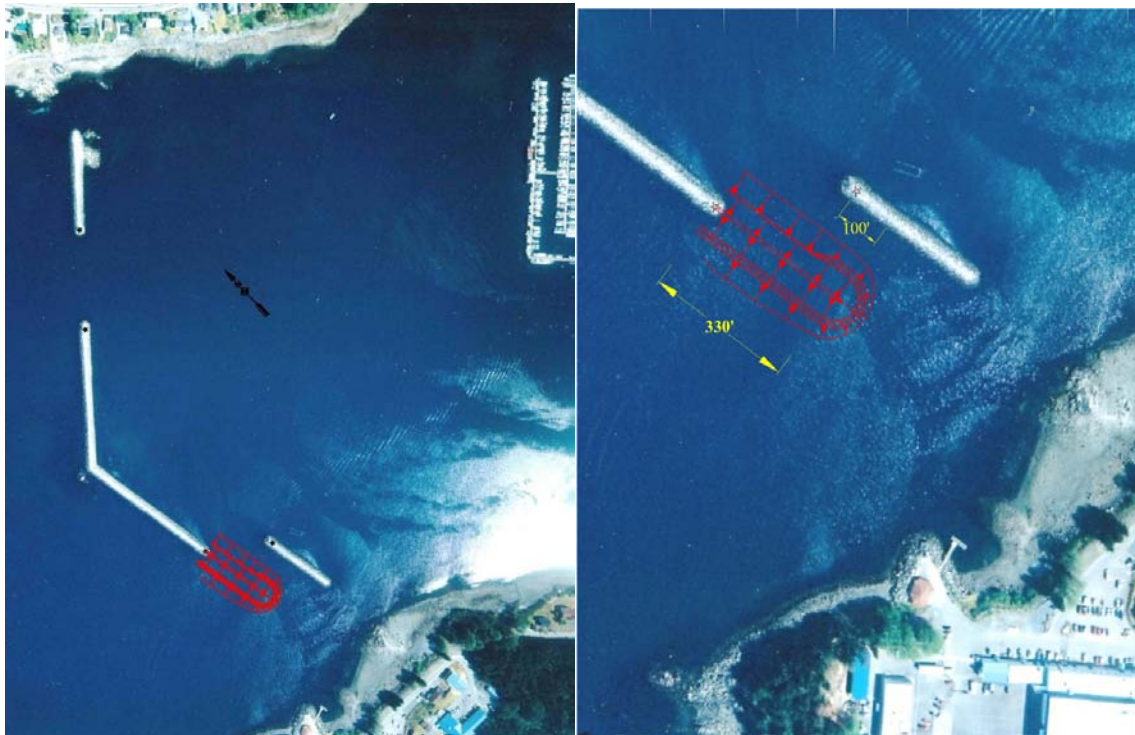
Figure 28. Plan 3. Breakwater overlap outside overall and close up view – drawing not to scale.
