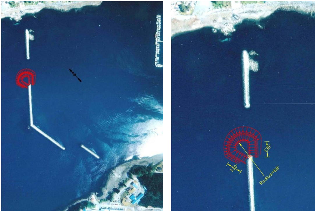
Figure 32. Plan 15 (bulbous head option). Bulbous head at the gap between the main and north breakwaters. Overall and close up views – drawing not to scale.
