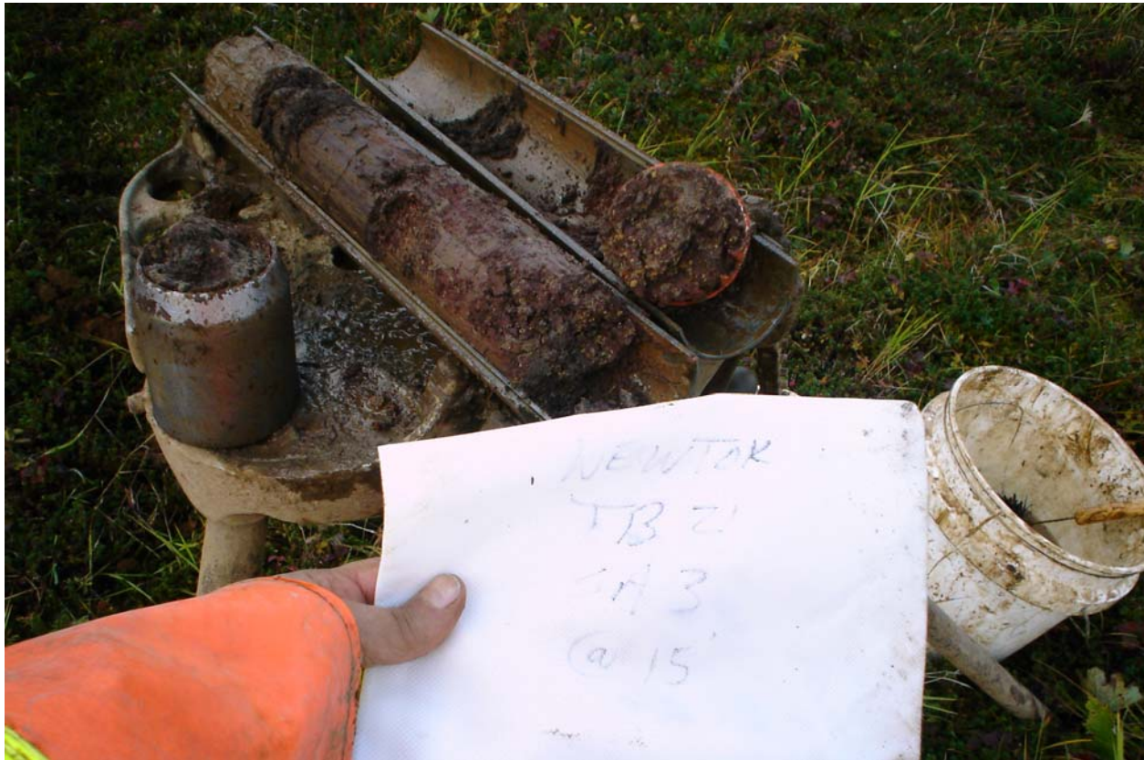
Photograph 2. Sample of material that is typical of the soil composed of residual basalt.
