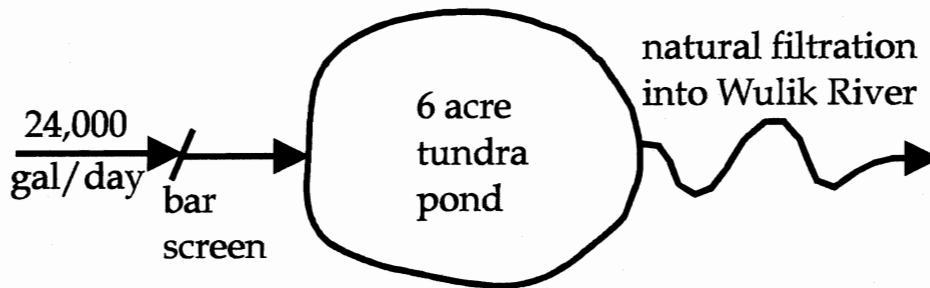
FIGURE H-3.--Schematic flow diagram for sewage treatment at Igrugaivik site.
