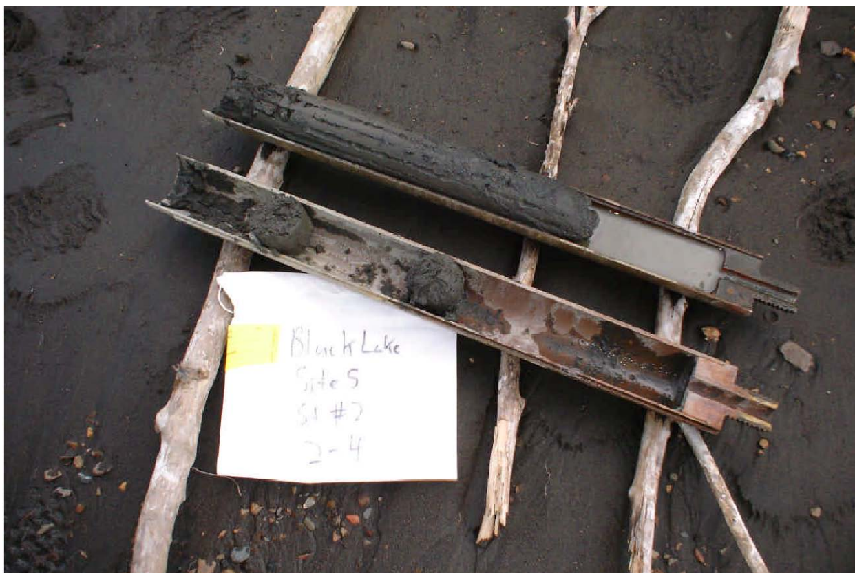
Figure 26. Sample from 24 to 48 inches below the channel bed at Core Site 5.
