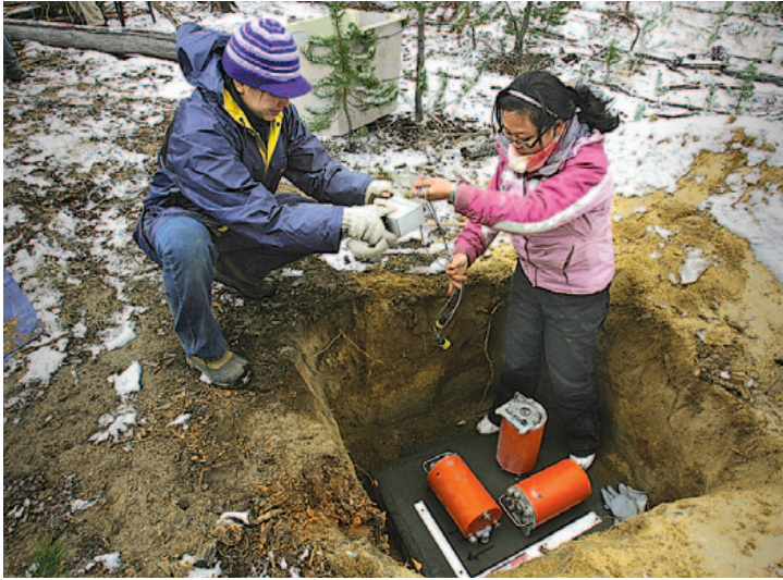
Livermore seismologist Dennise Templeton (left) and postdoctoral researcher Jingbo Wang install seismometers at AltaRock Energy's Davenport Newberry Enhanced Geothermal System Demonstration Site near Bend, Oregon. (Photo courtesy Pete Erickson/ The Bulletin .)
