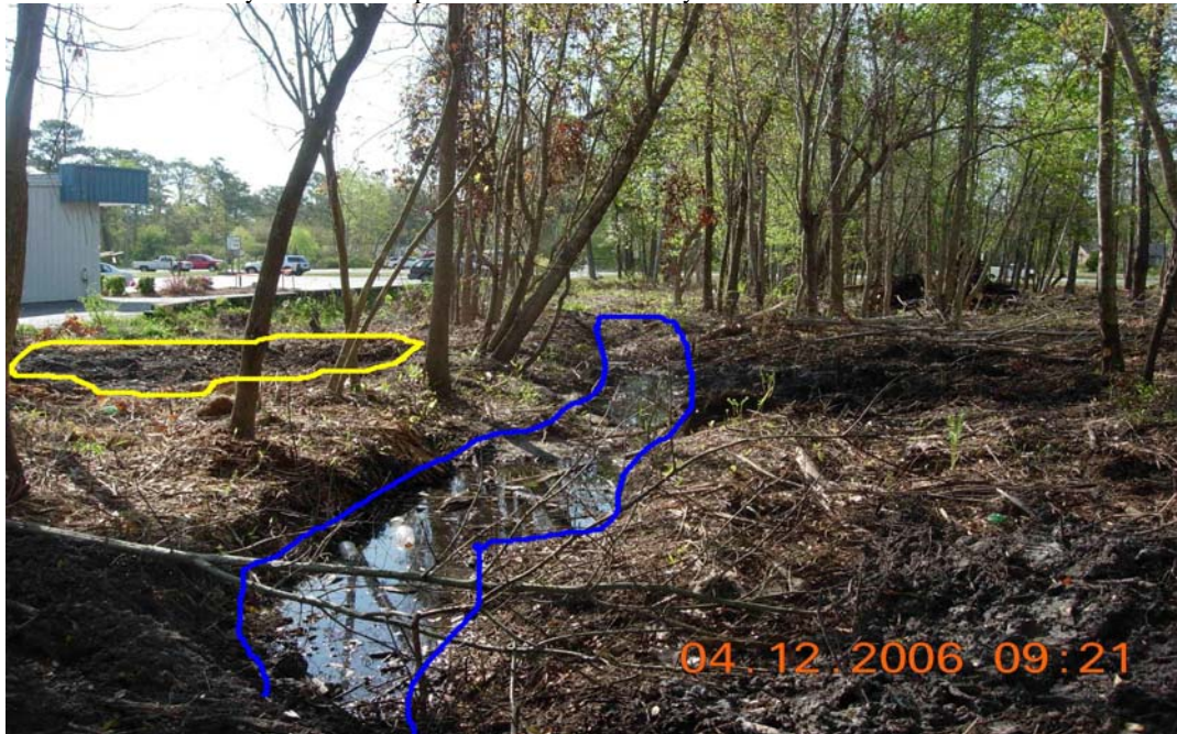
Photo 40: Adjacent wetland, South Atlantic Division. Wetland is marked in yellow and is separated from non-RPW by a man-made berm. Non-RPW marked in blue.
