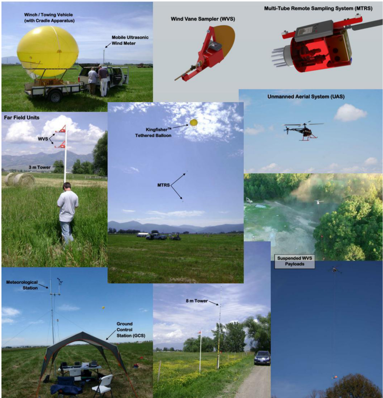
Figure 6: MTRS and WVS Systems for Atmospheric PFT Tracer Monitoring. (Pekney et al., 2011)
